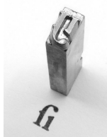
FIGURE 2. A ligature type and its printed image (Daniel Ullrich, Threedots, CC BY-SA 3.0, https://commons.wikimedia.org/w/index.php?curid=855947 )
